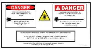
\*Caution - Use of controls or adjustments or performance of procedures other than those specified herein may result in hazardous radiation exposure.
